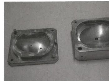
Figure 4: Mold for production of customized implant. CENTIMFE ©
